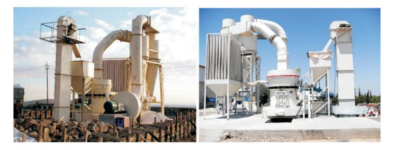
Powder grinding equipment is mainly used for grinding non-flammable and nonexplosive materials whose Moh's hardness is below 9.3 and humidity less than 6% such as cement, quartz, feldspar, barite, calcite, gypsum, limestone, dolomite, talc, marble,
