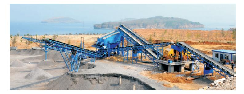
Stone crushing production line is mainly composed of vibrating feeder, jaw crusher, impact crusher, vibrating screen, belt conveyor and centralized electronic control. The designed output is 50-800t/h and cone crusher and dust removing equipment can be equipped to satisfy different processing needs of the customers.
